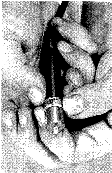
Figure 5-2. Unscrewing tip from probe. Notice little finger of hand holding cable, to withdraw inner part of probe from tip.
